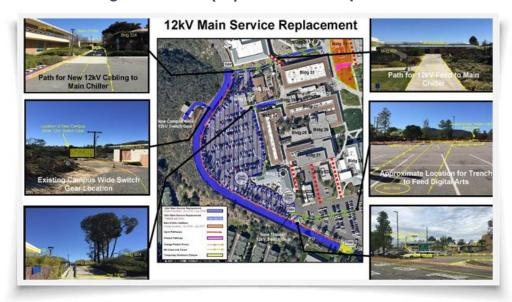
This project includes an expansion of electrical to service the Arts and Communications Complex, Teaching and Performance Theater, Building 31, and Main Chiller projects. In addition, new data, fire alarm and security low-voltage conduits will be installed. Sections of Grossmont College Dr. will receive repairs and repavement. Bid responses are currently under review and construction is anticipated to begin in June.
